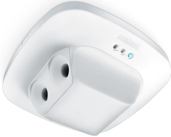
The US Hallway DCS is a digital (40kHz) ultrasonic technology occupancy sensor that utilizes STEINEL's state-of-the-art ultrasonic signal processing to provide superior stable volumetric bidirectional detection. The unique linear bidirectional coverage pattern is engineered specifically for hallways and applications requiring a true linear volumetric pattern of detection. This is an ideal hallway sensor for design and retrofit applications.
